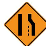
Advance Warning Signs shall be fluorescent Orange in color, with approved legends and shall be 48" X 48" in size. Wherever possible, the distance of the advance warning signs should be increased if the sight distance is restricted due to the presence of a vertical or horizontal curve.
